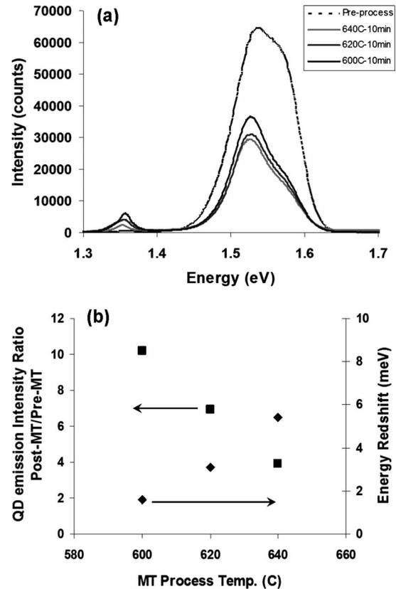
FIG. 3. Low temperature PL spectra of pre- and post-MBE mass transport processed samples (a) (excitation energy density of 100 W/cm<sup>2</sup>) and QD emission intensity ratio of post-MT/pre-MT and PL peak energy redshift depend on process temperature (b).
